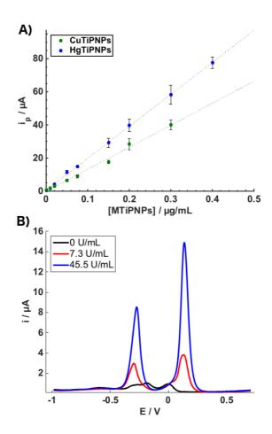
**Figure 3. A)** Calibration plots of the HgTiPNPs and CuTiPNPs. **B)** Electrochemical response of the proof-of-concept multiplexing biosensor using HgTiPNPs and CuTiPNPs as detection label.
