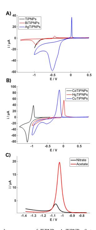
**Figure 1. A)** Cyclic voltammograms of TiPNPs, AgTiPNPs (between +0.5 and -1.0 V) and BiTiPNPs (between -1.4 V to +0.5 V with a deposition step at -1.4 V for 30 s). **B)** Cyclic voltammograms of CdTiPNPs (between -0.4 and -1.4 V), HgTiPNPs and CuTiPNPs (between +0.8 V and -1.0 V) in 0.1 M pH 4.5 acetate buffer. **C)** Square-wave voltammetry of CdTiPNPs synthesized by using a nitrate or acetate salt during the cation-exchange reaction.
