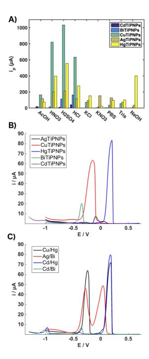
**Figure 2. A)** Peak currents of the anodic stripping process for the different MTiPNPs using different electrolytic media. Concentration of electrolytes was 0.1 M. **B)** Square-wave voltammetry of the different MTiPNPs in 0.1 M H<sub>2</sub>SO<sub>4</sub>. **C)** Square-wave voltammetry of several MTiPNPs binary mixtures in 0.1 M H<sub>2</sub>SO<sub>4</sub>.
