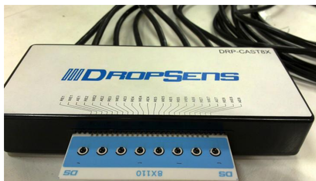
Figure S1. Image of the 8-channel screen-printed electrochemical array and the corresponding connector to the Dropsens \mu Stat 8000 potentiostat.
