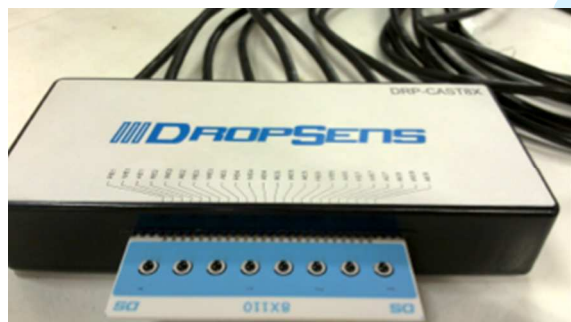
Fig. 1. Image of an 8-channel electrochemical screen-printed array.
